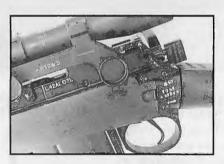
This L42A1 sniper rifle was converted to caliber 7.62x51mm NATO in 1971 at the Royal Small Arms Factory, Enfield Lock, from a No. 4 Mk I (T) SMLE originally manufactured in 1943. Note that the scope was manufactured in 1945 and that the scope mount carries the rifle's serial number.
